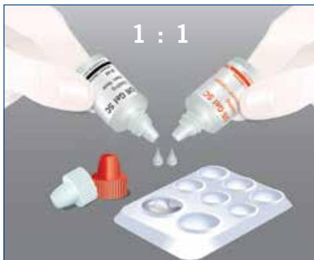
Mix Glazing base and catalyst homogeneously in a 1:1 ratio
