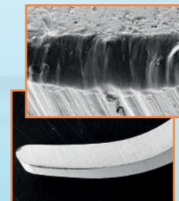
Cutting edge of a typical non-coated curette and the magnification of the edge after the test.
