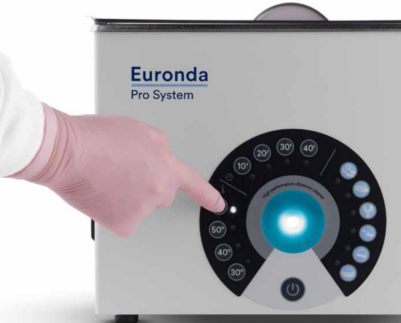
There are two operational modes, allowing users to choose one of the 6 preset cycles (instruments, burs, impression trays, cement removal, plaster removal, and prostheses) or run a free cycle at a temperature between 30°C and 60°C, with a duration between 10 and 40 minutes. There are 4 different operating stages in the 6 preset cycles: Degas, Boost, Normal and Sweep.
